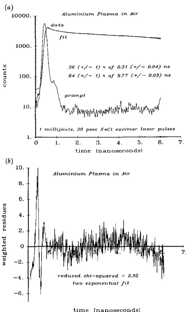
**Figure 5.** (a) The luminescence decay profile from a laser ablation plasma formed by focusing 1.0 mJ, 35 ps pulses at 308 nm onto an aluminium target in air shows components at 0.31 and 9.77 ns. (b) The plot of the weighted residues in this case exhibits large deviations near the prompt and a non-random trend which suggests the presence of a third component.
