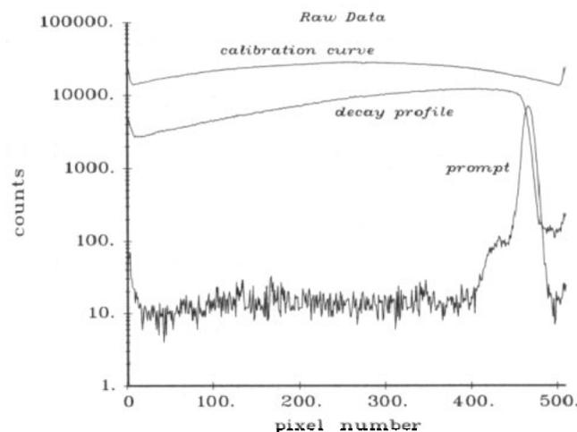
**Figure 3.** The calibration curve, used to correct for an overall non-linearity of response with time, was obtained by collecting light from a steady source. The uncorrected data for one of the fluorescence decay profiles and for the prompt function are also shown on this semilogarithmic plot. The channel number corresponds to time increasing from right to left (12.1 ps per channel).
