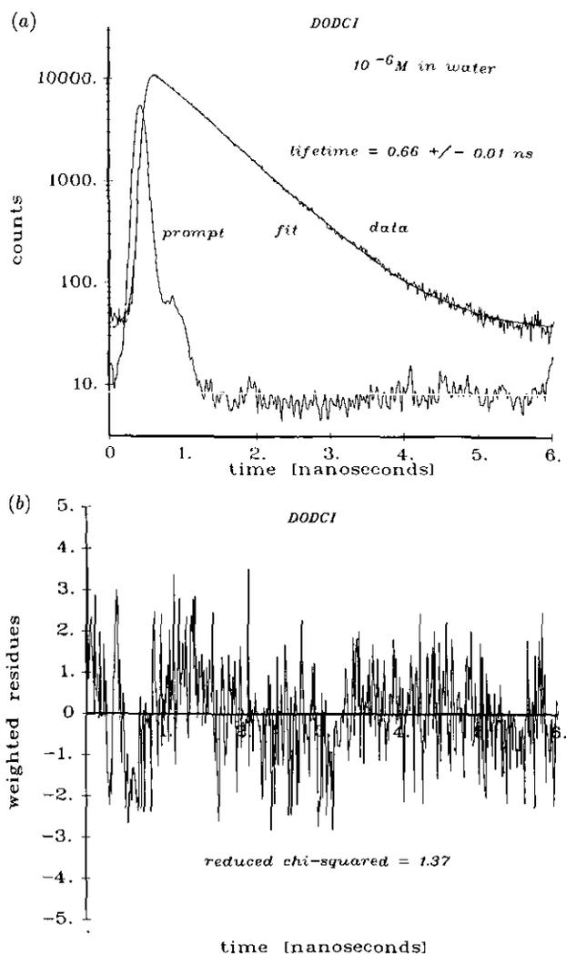
**Figure 4.** (a) The recalibrated decay profile from DODCI dye solution excited by the attenuated picosecond excimer laser pulses yields a single exponential lifetime of 0.66 ns. (b) The weighted residues for the fit are evenly distributed about zero, although  $\chi^2 = 1.37$ , possibly indicating the presence of other random errors.
