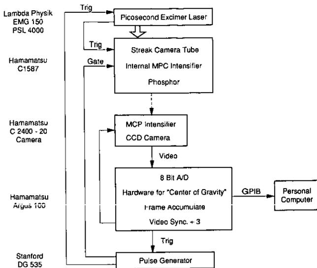
**Figure 1.** Configuration of instruments used to achieve time correlated photon counting with a streak camera and 10 Hz picosecond excimer laser.
