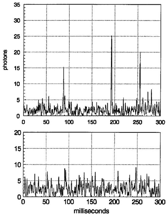
Fig. 7. Photon-burst signals from S-101 and water in the simple flow cell.
