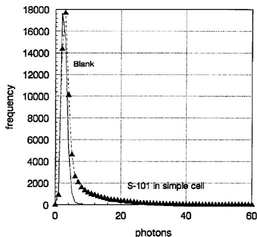
Fig. 8. Histograms of burst amplitudes from S-101 and water in the simple flow cell.
