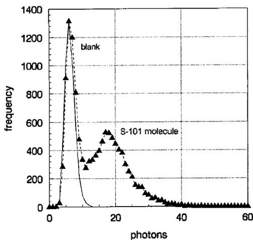
Fig. 11. Histograms of burst amplitudes from S-101 and blank with the capillary injection system.
