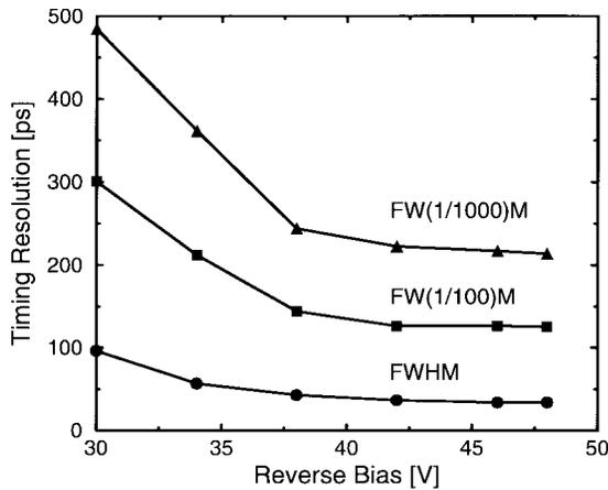
Fig. 4. Experimental values of the IRF width of the DJ-SPAD at various levels (1/2, 1/100, and 1/1000 of the maximum) with increasing negative bias voltage.
