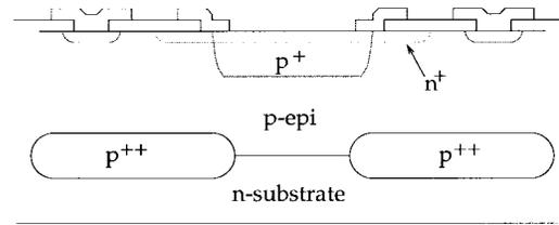
Fig. 1. Schematic cross section of the DJ-SPAD device.
