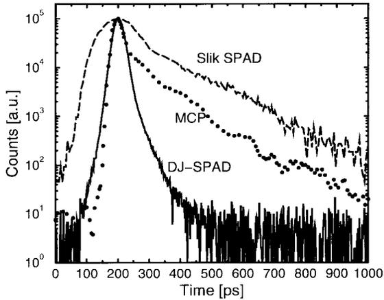
Fig. 3. IRF of the DJ-SPAD (operating with 21-V excess bias voltage above the breakdown voltage of 27 V). For comparison, measured IRF's for a Hamamatsu R2809U MCP and for an EG&G SLiK SPAD (operating with 40-V excess bias voltage above the breakdown voltage of 410 V) are shown, normalized to the same peak height.
