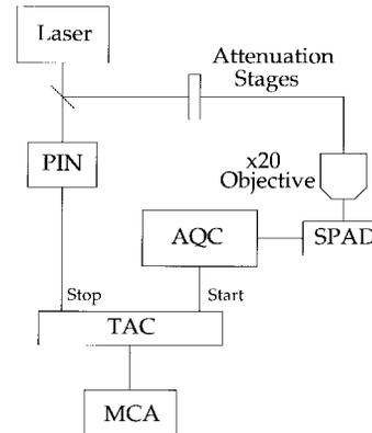
Fig. 2. Experimental setup for measuring the timing resolution.
