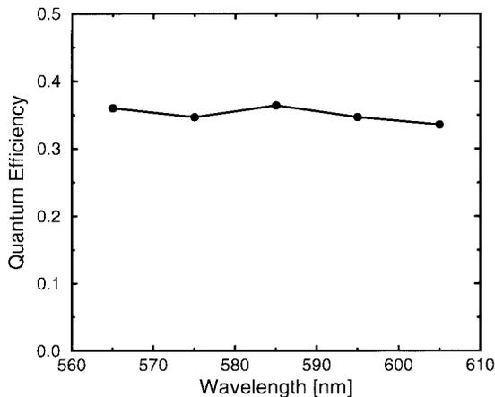
Fig. 5. Measured QE of the DJ-SPAD.
