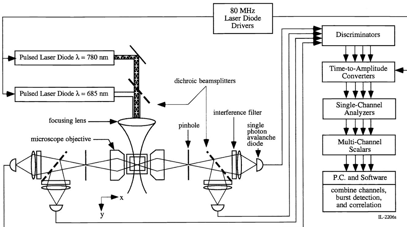
**Figure 1.** Experimental set-up to be modeled.
