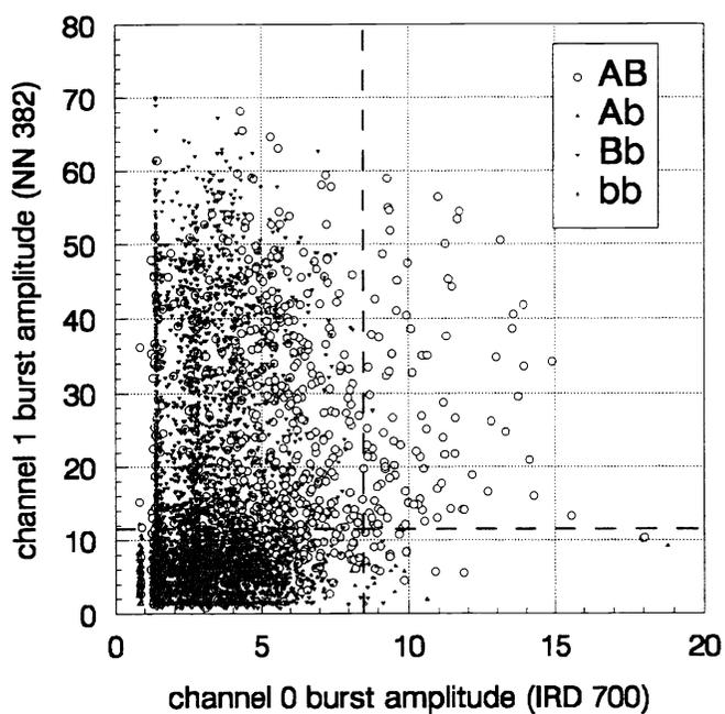
**Figure 3.** Plot of amplitudes of simultaneously detected bursts due to the following: AB: both fluorophores; Ab: IRD 700 in channel 0 and background in channel 1; Bb NN382 in channel 1 and background in channel 0; bb: background in both channels.
