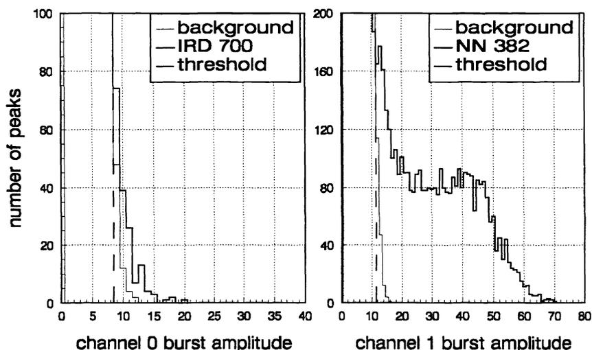
**Figure 2.** Histograms of Gaussian weighted sliding sum peak amplitudes, due to background fluctuations and passage of (a) IRD 700 fluorophores, and (b) NN 382 fluorophores.
